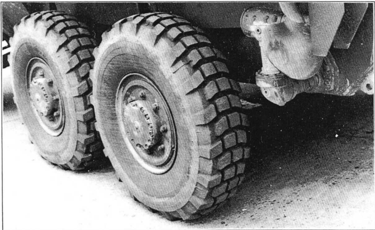
Figure 8-4-3 Tread Design of a Mounted Tire Sculptures de semelle d'un pneu monté
