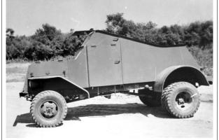
**Remarks**: A private venture by Chrysler to produce an inexpensive and quick armored vehicle on an existing commercial chassis. The armored body was bolted to the top of a Dodge 1/2-ton 4x4 chassis. The vehicle proved to be to narrow and had a very high center of gravity. The same vehicle was later modified with an armored cab and a cargo body at the rear, but no orders were ever placed.
