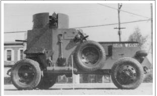
**Remarks**: QMC and Franklin, 4x4, interchangeable truck or armored bodies, 6 built. Armament (1) .50 caliber HMG and two .30 caliber light machine guns. Engine, Franklin 6-cyl. This car had an unloaded weight of 7.200 pounds, a road speed of 60 mph (64 km/h) an armor thickness of .19 inches (4.82 mm), carried a crew of four men and was armed with one .50 caliber and two .30 caliber machine guns. It had single front and dual rear wheels with front wheel drive.
