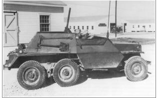
**Remarks**: Using the same extended 1/4-ton chassis as on the 37mm Gun Motor Carriage, T14, development of the scout car started in early 1942. While the Tank Destroyer Command and the Special Armored Vehicle Board both recommended standardization late in the same year, there
