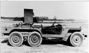
Above: One of the original two, T-14 37mm GMC with early Willys Model MB "slat" grille. Besides a change of angle in the steering wheel, the whole steering unit had been moved approximately 10-inches to the outside (left). (Photo: US Army) Remarks: At least two slat-grille T-14s were completed
