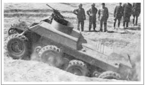
Remarks: A private venture by the Trackless Tank Corporation, the vehicle was tested by the Armored Board for use as an armored car, rather than as a tank. Chain drive was used to the last three axles, the front axle being used for steering. While no orders were awarded for the Trackless Tank, it did directly lead to the T13 Armored Car.
