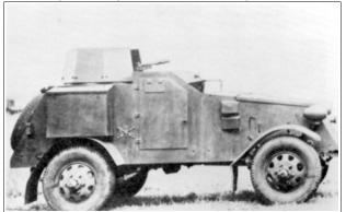
Remarks: Fitted to a Franklin chassis with an air-cooled engine, the early T6 had a body very similar to that of the T2E3 Armored Car. Biggest visual difference is the set of dual tires at the rear.
