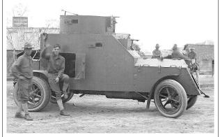
Above: Armored Motor Car, No. 2. Photo was taken while on the Mexican Border. (Photo: Author's collection) Vehicle Data: Weight empty (est), 8,000 lbs (3632 kgs). Weight loaded, (est), 9000 lbs (4086 kgs). Length, 172 in
