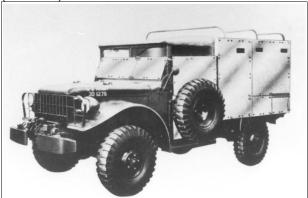
Above: M37B1 <sup>3</sup>/<sub>4</sub>-ton Truck with Materials Research Agency designed armored panels. (Photo: US Army).
