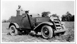
Remarks: One vehicle (W-1300) was further modified to T2E3 status, with a revised turret and a stepped closed top at the rear. The machine gun mount allowed for a relatively high angle of fire. Armament was one .30 caliber air-cooled machine gun.
