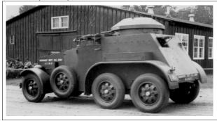
Above: T4 6x4 Armored Car. (Photo: US Army) Remarks: Designed and built by James Cunningham Sons and Company, two T4 Armored Cars were completed and tested until 1934 when the design was type classified as the M1 Armored Car. After classification, an additional ten cars were completed. While the cars' performance on hard surfaces was adequate, the non-driving front axle and length of the vehicle (even with the spare wheels able to rotate on stub axles) made cross-country travel marginal at best.
