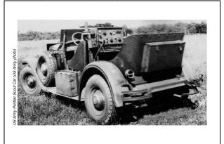
Remarks: Pontiac chassis, open crew compartment with armored radiator and windshield. Later modified with pneumatic tires on passenger vehicle rims, wide, rather than bucket seats, and an SCR-163 Radio Set facing the rear seats. Circa 1928-1932.
