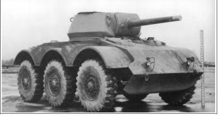
**Remarks**: With the closing of the T19 Armored Car project, the only T19E1 pilot vehicle was modified at the request of Tank Destroyer Command. The 75mm gun M3 was mounted in an open circular turret and fitted to the chassis as the Carriage, Motor, 75-mm Gun, T66. The circular turret was later replaced with a more oval shape allowing extra room for the crew to function. Although the vehicle showed promise, Tank Destroyer Command lost interest and the project was canceled in November of 1942.
