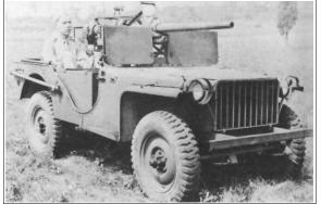
Remarks: The T2E1 used a Bantam chassis, but with out the major changes of the T2. On this vehicle, the 37mm gun was fitted to fire to the front. No production undertaken.
