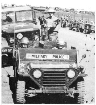
Above: M151A1 with the first semi-standard armor kit as specified and supplied from the states. (Photo: US Army) **Remarks**: The first "standard" armor kit was a simple box of .25 inch (6.35mm) armor plate cut to be welded/bolted to the actual vehicle body. A low plate across the front of the vehicle protecting the driver and passenger, plus a simple box was the first attempt under the, "something is better than nothing" approach.
