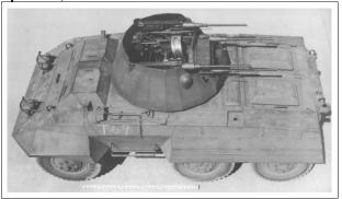
**Remarks**: Based on M8 Armored Car 6x6 chassis. A quad .50 caliber HMG mount was fitted, but no improvement was found over the then standard M16 SPAA half-track. Because the M16 was already in production, no series order for the T69 was issued.
