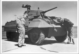
Above: M8 Light Armored Car pre-production vehicle. (US Armv) Remarks: Type classified as the M8 Light Armored Car, the T22E2 was the first production version (of three). The T22E2 included a redesigned driver's compartment, addition of armored sponsons to hold the required radios, the addition of sand shields over the wheels, and finally changes to the turret top to improve visibility for the commander and gunner. After a final redesign, this vehicle became the M8 Light Armored Car, circa 1942.
