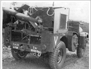
Above: M38A1 fitted with three French SS10 Anti-tank Missiles. (Photo: US Army)
