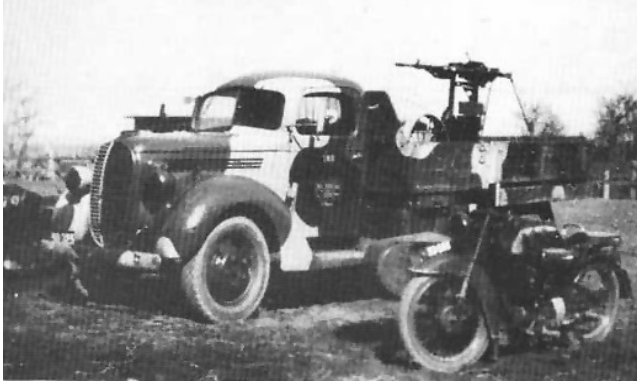
Above: Ford commercial two-axle medium truck with 20mm AA gun mounted in the rear.
