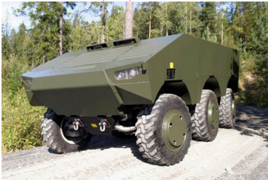
Above the SEP with the suspension raised. (Photo: BAE Systems Hagglunds)
