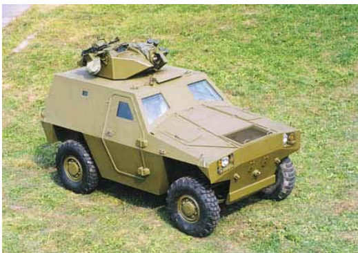
Above: Aligator 4x4 ORP with MOWAG MBK2 turret. (Photo: Kerrametal)
