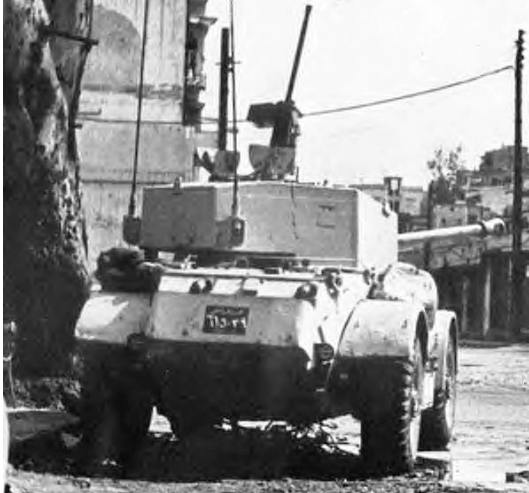
Above: Lebanese Army T17E1 with AEC Mk III turret. (Photo: Author's collection).
