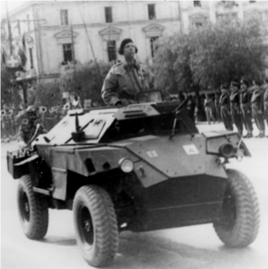
Above: A Humber Scout Car Mk I, as supplied from British stocks after WWII. (Photo: T. Metsovitis)
