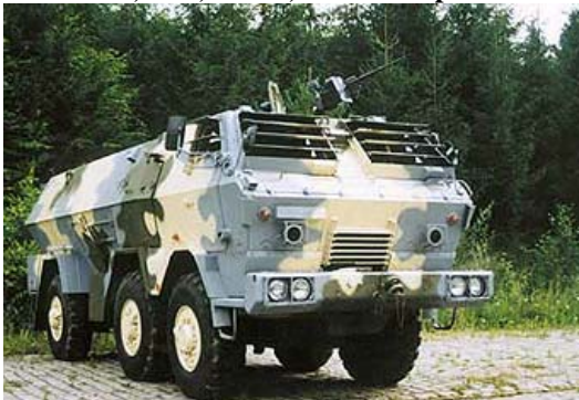
Above: Tatravan MOD with APC rear compartment. (Photo: Kerametal)
