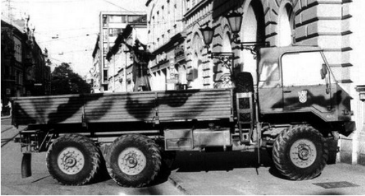
Above: Unarmored Croatian TAM 150 with pedestal mounted 20mm cannon in the back.
