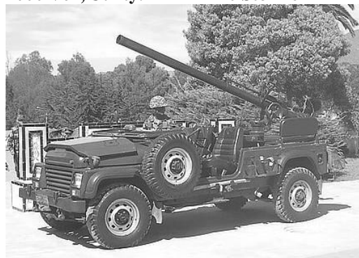
Above: AIL M240 Stormer fitted with a 105mm Recoilless Rifle. (Photo: Ejército de Chile).
