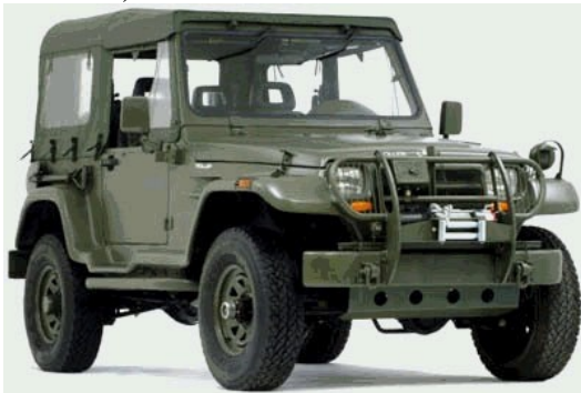
Above: Troller T4-M with canvas top but without roll-bars installed. (Photo: Troller Veiculos Especiais s.a.)
