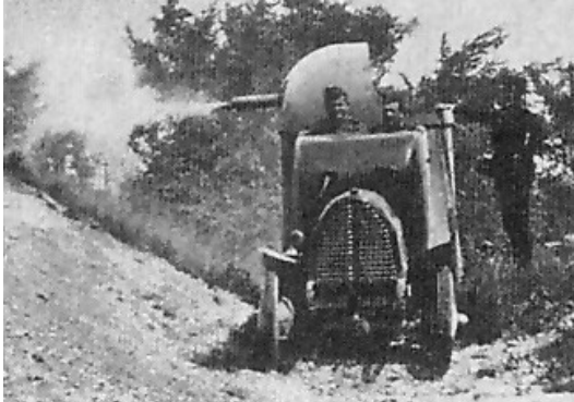
Above: Austro-Daimler as modified with the rear of the turret cut-away for better ventilation and vision. (Photo: Author's collection).
