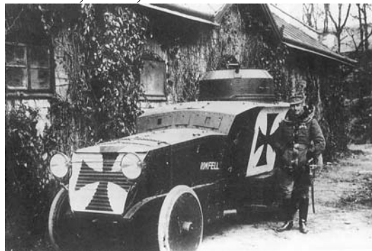
Above: The original Romfell Model 1915 with a Mercedes chassis and engine; power was supplied to the rear wheels via chain drive. (Photo: Author's collection)
