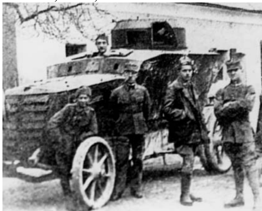
Above: The Romfell Model 1917, the most obvious difference from the 1915 version, is the front axle and changes in radiator armor. (Photo: Author's collection)
