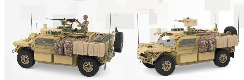
Manned or remote weapon station capable from 7.62mm to .50 caliber armament.
