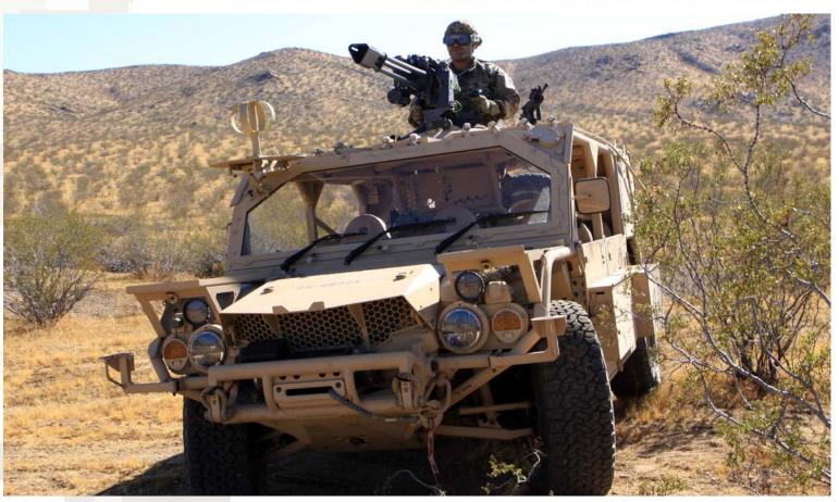
The Flyer® 72 is a non-developmental item, purpose-built, lightweight vehicle designed to meet complex mission sets. Selected by the U.S. Special Operations Command (USSOCOM) as the vehicle of choice for their Ground Mobility I.I (GMV I.I) program, at 72" wide it is capable of internal transport in the CH-47 and C-130 aircraft.
