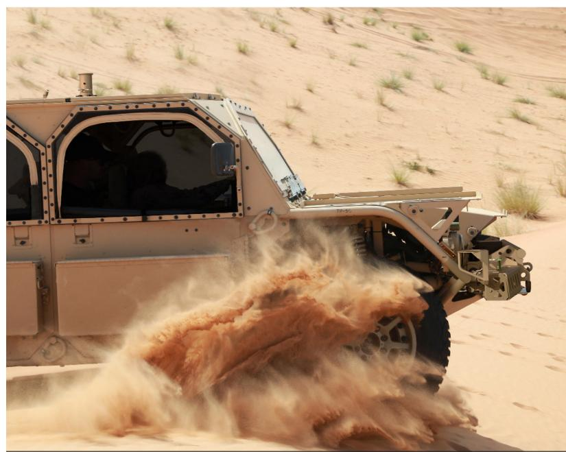
The Flyer<sup>®</sup> 72 is a non-developmental item, purpose-builightweight vehicle designed to meet complex mission set Selected by the U.S. Special Operations Command (USSOCOM as the vehicle of choice for their Ground Mobility 1.1 (GMV 1 program, at 72" wide it is capable of internal transport in the CH-47 and C-130 aircraft.
