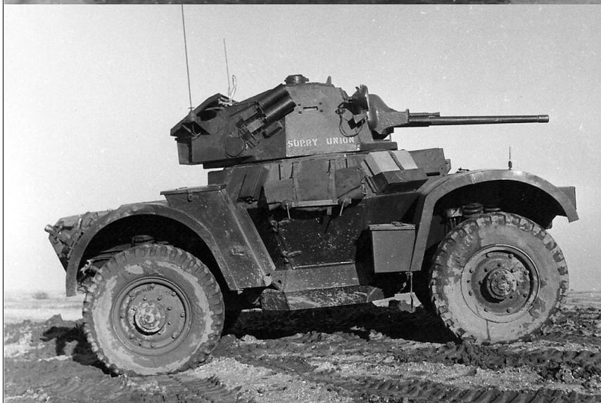
Above: Daimler Mk II Armored Car, the most obvious difference between the Mk I and Mk II is the rectangular mantlet on the Mark I and a more rounded shape on the Mk II.
