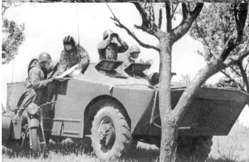
Above: (Top) East Germany (DDR) BRDM-1 M1959 with a single pintle mount light machine gun. (Bottom) An early Soviet Army BRDM-1U M1958 Command Vehicle.
