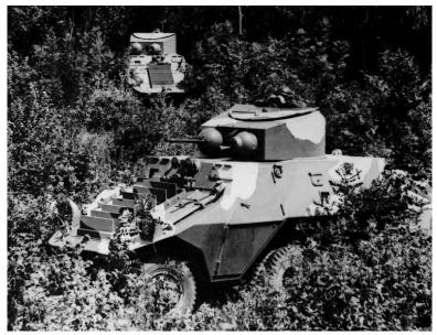
Remarks: The ADGZ was developed and put into service by Austria with production vehicles produced between 1935 and 1937, with the original prototypes appearing in 1931. Protected by .43 inch (11 mm) of armor, two drivers were equipped with duplicated controls allowing full-speed in three gears in either direction.Used by the Austrian and later German forces (mainly SS units), at least one vehicle was captured and put into service
